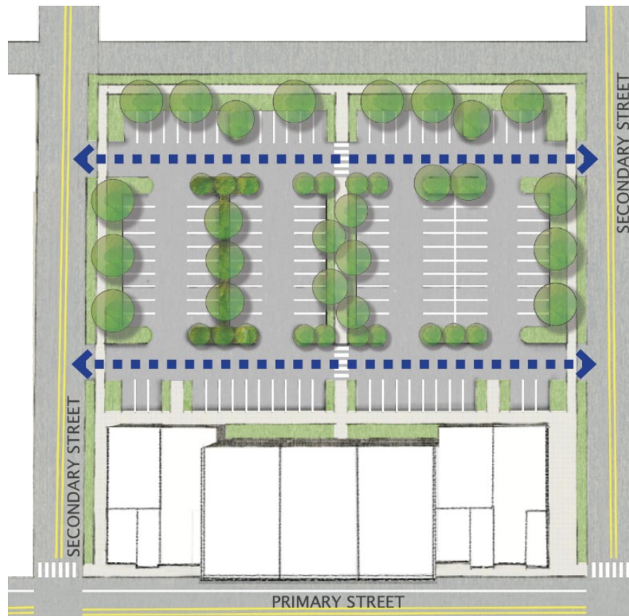
FIGURE 30.2: Vehicular Cross Access
